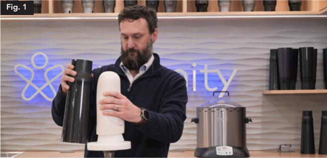
Proper sizing of the Preform is critical for successfully fabricating the XtremityTT Socket. Refer to the sizing chart for proper size selection.
